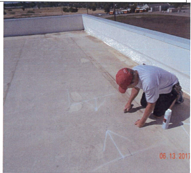
32b-west-P1716_20170613_JG01-039 Example of "wet reading" area
