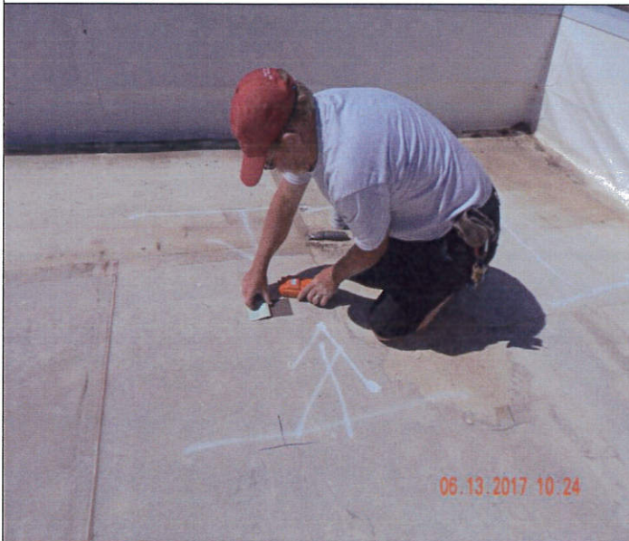
36a-west-P1716_20170613_JG01-044 West gym - Example of moisture reading area
