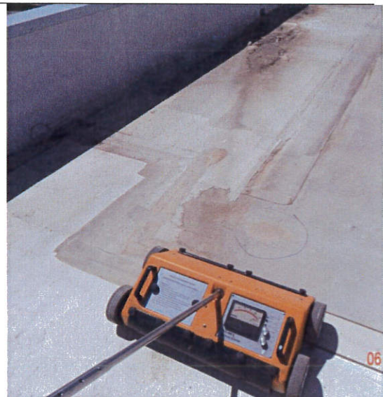
39b-east-P1716_20170613_JG01-054 Example of Tramex readings - East
