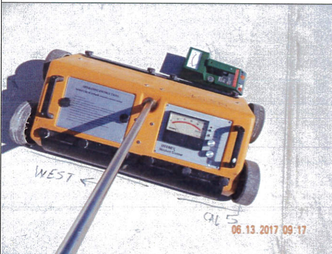
32a-west-P1716_20170613_JG01-027 Tramex device – dial is calibrated
