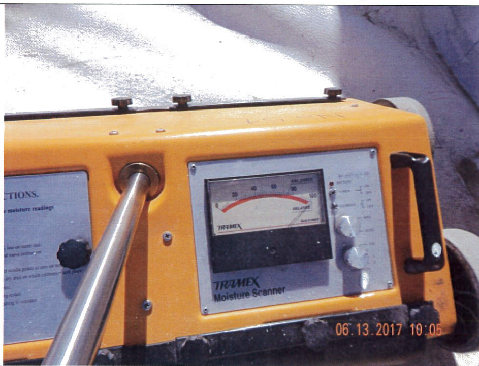
34-west-P1716_20170613_JG01-032 Example of Tramex Moisture Scanner – 100 reading
